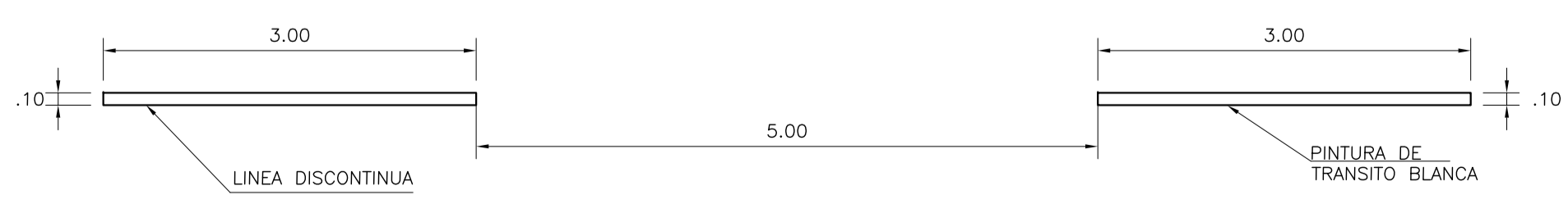
LINEA DISCONTINUA – DIVISION DE CARRIL 3mts. ESC: 1/50
